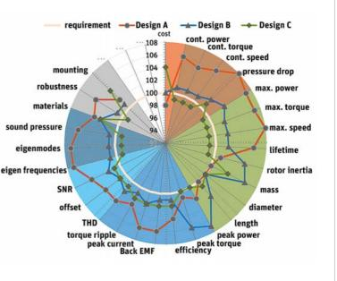
A radar chart illustrates three design concepts and how well they meet customer requirements.
