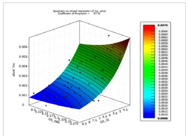
Fig. 4b: Strain amplitude as function of strut length (SL) and strut thickness (SBK)
