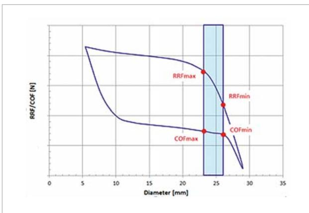
Fig. 3b: Evaluation points of the Nitinol curve
