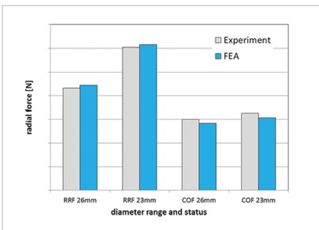
Fig. 3a: Comparison of experimental vs numerical radial force results for an exemplified stent design in a 23mm and 26mm vessel model
