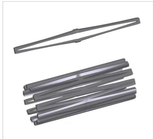
Fig. 1: Single diamond cell and the reconstruction of a 360° full stent model with 12 single cells
